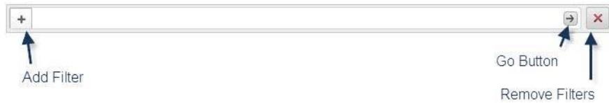
The Filter Bar is at the top of the Report. It contains **Add Filter (+)** for adding filters and a **Go** button to apply filters, as well as the **Clear Filter** button to clear all filters.
